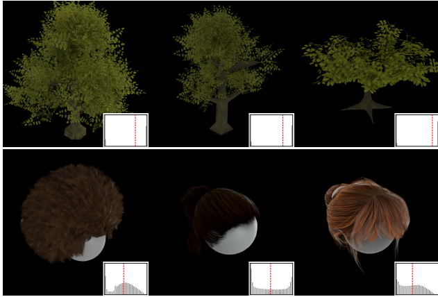
Fig. 6. Distributions of our kernels on different types of scenes. From the top row to bottom, vegetation and hair scenes. Each inset shows the corresponding histogram of d_1 (Eq. (6)) of our learned kernels, with the red dotted line indicating the mean; the range of the horizontal axis is [0, 1] .
